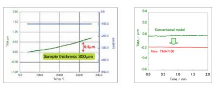
When measuring very stiff samples or thin films, the amount of expansion and compression is tiny. Within this range, there is always the risk of losing the signal within the baseline noise level of the instrument. To
