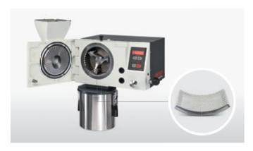
**Clean design:** The P-16's grinding chamber is designed so that it collects virtually no residue. Its impact plates and the bottom sieve can be removed in a few simple steps. Perfect conditions for quick, easy cleaning.
