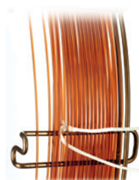
Integra-Guard® Built-In Guard Column
