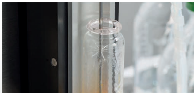
Rinsing of sample vial for quantitative transfer
