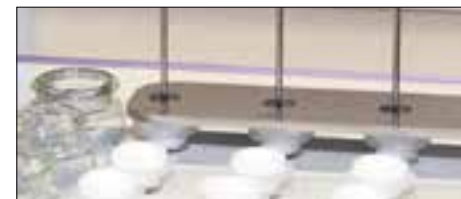
Three needles work on the columns in parallel. Three-fold sample throughput.
