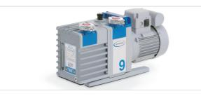
Vacuum pump, RZ 9 140 L/min and 8,6 m3/hour. The ultimate vacuum is 0,0002 mBar. Included is the oil mist filter – art no.: 7001201070.
