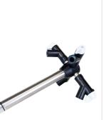
Manifold 4 Basic Manifold Basic with 4 rubber valves 3/4 inch for freeze drying in flasks. (Can be extended with the addition of Manifold 4 Extension).
