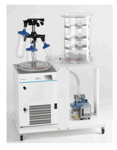
If the condenser temperature is near to the freezing point of the sample, then the freeze drying cycle times are extended.
