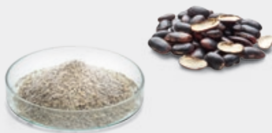
Homogeneous sample: Beans before and after grinding with the Variable Speed Rotor Mill PULVERISETTE 14
