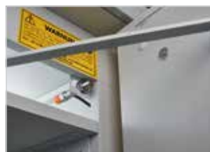
Status query door opening This sensor can provide an easy way to monitor the status of the door (open/closed).
