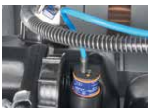
Level monitor with control module to warn about overfilling.
