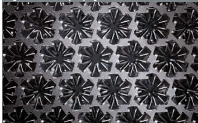
Figure 9 - StarCell pumping element
