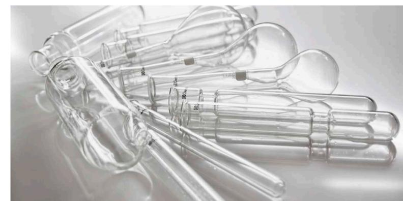
Digestion tubes and Kjeldahl flasks
